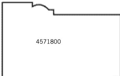
A thick molding providing a surface for brick or other siding to butt against. This design allows a brick molding up to 2" wide x 1-1/4" thick to be produced. Profiles shown at approximately 100% of actual size.
