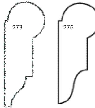
This profile is used to support hooks for picture frames. Installed around the perimeter of a room approximately 1-1/2" below the ceiling line. Profiles shown at approximately 100% of actual size.
