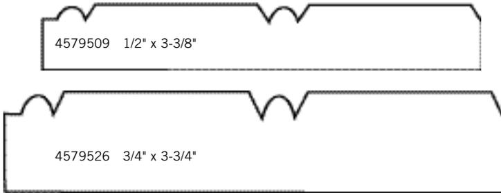
Wainscot molding is very popular in remodeling projects or new construction because of the warmth it imparts to a room. After installation, cap off your new wainscot with your choice of cap moldings. Available in two different sizes to suit your needs. Each shown at approx. 100% of actual size.
