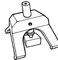
Take readings on the left and right side of the planer knives and the adjustable floating top pin will indicate alignment. An economical alternative to more expensive gauges. # 4501960
