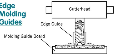
Use the optional edge molding guides when molding profiles such as tongue and groove patterns. Made from heavy gauge formed steel. Zinc plated to guard against corrosion. Four required. # 4509492
