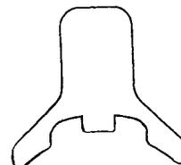
This simple gauge straddles the top of the cutterhead over the planer knives. Simply raise the knife until it makes contact with the gauge. Instructions are included. # MGA-B14D
